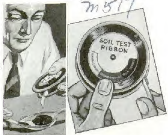
Paper ribbon shows whether soil is acid or alkaline
